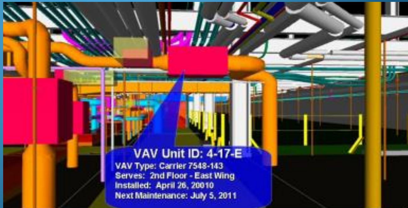
Figure 4 - Maintenance Management, University of Colorado Lab RC-II
